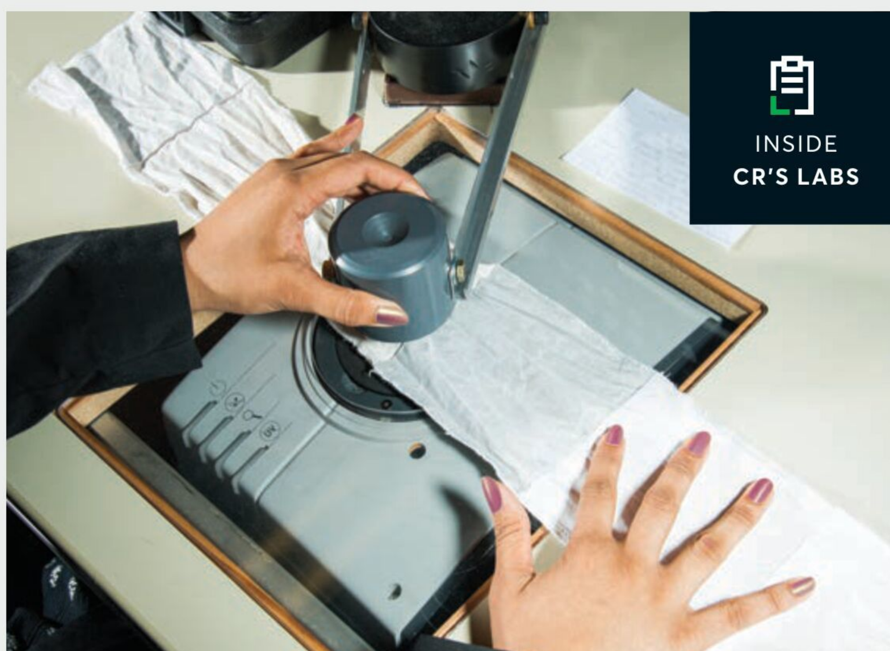
We use a spectrophotometer (a machine that measures color intensity) to analyze equally stained fabric swatches, before laundering and after. The lighter the stain after washing, the higher the cleaning score.
